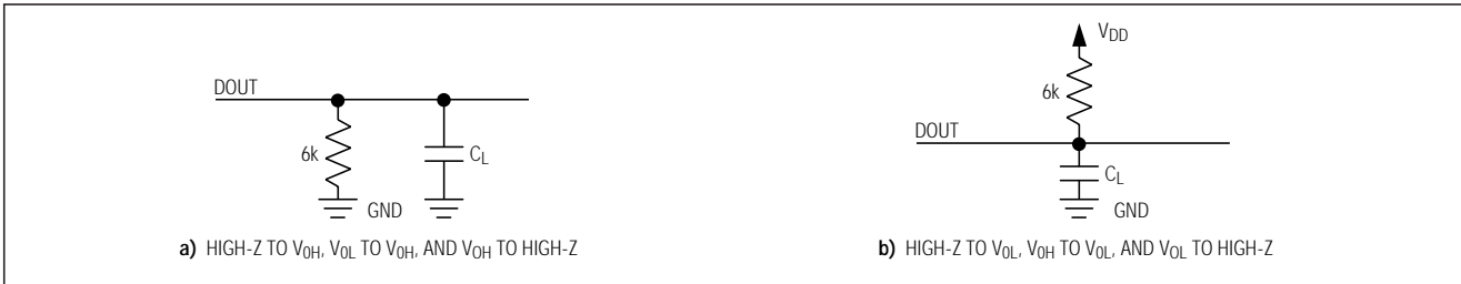
Figure 1. Load Circuits for Enable and Disable Time
